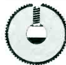
How shaft is positioned for set-screw knob.
