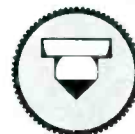
Shaft position in knob requiring 1/32" flat.
