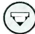
Shaft position in knob requiring 3/32" flat.
