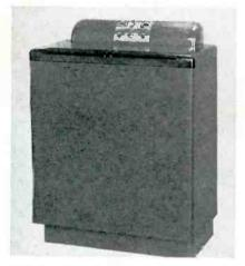
GENERAL ELECTRIC—Type FB-50 has gross Btu capacity of 6600. Room air circulation 200 c.f.m. Measures 25½ by 39½ by 18 1/16 inches. It is equipped with a modern control panel of dashboard style with indicating pilot light
