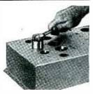
Here's a handy tool to help the radio worker save many hours of work when cutting holes for sockets, plugs, connectors, and other receptacles in radio chassis. A cap screw is inserted in a small drilled hole, and the punch is easily forced into the die by  $\boldsymbol{\alpha}$  few turns of the cap screw with an ordinary wrench. Smooth holes, requiring no filing or reaming, can be cut in metal up to 1/8-inch thick in 11/2 minutes or less.
