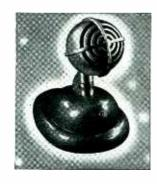
SHURE MICROPHONE, "Uniplex" Cardiold crystal cuts down room noise pick-up. Model 730S has built-in r.f. filter which protects against burnouts. Output level—33 db. below I volt for 10 bar speech signal. Swivel head. Satin chrome finish. Diameter 31/6 inch. Depth 31/6 inch. Complete with 7 ft. super-shielded cable. Available in Model 730SH at \$32.50 list; also in Model 730S, complete with desk mount, at \$35.50 list. Shure Bros., Microphone Headquarters, 225 W. Huron St., Chicago, III.
