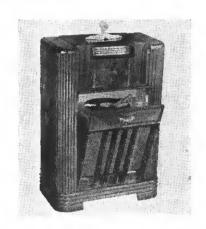
PHILCO 695-P Farm radio-phonograph designed for unwired homes. Receiver has 5 tubes and phonograph plays 10 or 12-inch records through a 1½ volt farm radio circuit. The filt-front console cabinet measures 37 high, 24½ wide and 13 inches deep. Philco Radio & Tele. Corp., Philadelphia, Pa.
