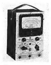
This Junior Voltohmyst, an electronic voltmeter-ohmmeter, provides for the complete meter overload protection on the DC voltage and ohm scales. No damage can be done if the probe slips to a high voltage point when a low DC voltage is being measured. DC voltmeter circuit has 6 ranges 0 to 3, 10, 30, 100, 300 and 1000 volts. AC voltage measurements on five scales 0 to 10, 30, 100, 300, and 1000. List price, \$34,95. RCA Mfg. Co., Camden, N. J.
