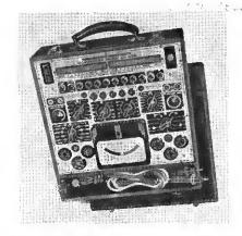
PRECISION 954 This combination dynamic mutual conductance type tube tester and 37 range ac-dc multi-range set tester is a complete compact unit. 20,000 ohms per volt including ranges of 6,000 volts ac-dc; 60 microamperes; 12 amperes and 60 megohms. Available in four models. Precision Apparatus Co., 647 Kent Avenue, Brooklyn, N. Y.
