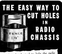
Here's a handy tool to help the radio worker save many hours of work when cutting holes for sockets, plugs, connectors, and meter holes in radio chassis. No tedious drilling, reaming, or filing is necessary. A cap screw is inserted in a small drilled hole, and the punch is easily forced into the die by a few turns of the cap screw with an ordinary wrench. Ten punches are available for cutting 34, 78, 1, 118, 153, 136, 114, 138, 112 and 214 inch holes. Write for more information.
