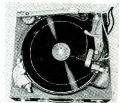
PRESTO 400A This blower system eliminates one of the commonest hazards of instantaneous recording. It directs a tiny blast of air across the surface of the disc just behind the cutting head which throws the waste thread to the center of the disc. The blower consists of an electric motor direct coupled to a positive pressure air pump. It includes a 6-foot rubber hose with metal nozzle. Price $75.00. Presto Recording Corp., 242 W. 55th St., New York, N. Y.
