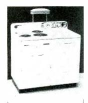
ELECTRIC RANGE—Equipped with oven; 2 utility drawers; 3 variable speed units; cooker, deep fry basket, variable heat; new smokeless broiler grill; illuminated dial on oven control; selective switch for time control of oven or outlet; deluxe warming drawer, lower right, with signal light and automatic temperature limiting control; automatic interior oven light, 25 watts. Landers, Frary and Clark, New Britain, Conn.
