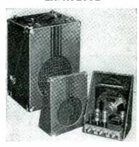
SOUND SYSTEM—Complete beam power amplifier, 2 speakers, cables, plugs and airplane-luggage carrying case. Provides 15 watts output; 113 db. gain; facilities for mixing and fading 3 channels; universal output impedance from 2 to 500 ohms. Radio Wire Television, Inc., 100 Sixth Ave., New York, N. Y.
