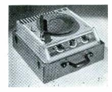
SOUND SYSTEM—A 20 watt combination 6 volt d.c. and 115 volt a.c. system in handsome tweed carrying case. Provision is made for either microphone or phono reproduction. Output is variable for various speaker loads. Erwood Sound Equipment Co., 224 W. Huron St., Chicago, III.
