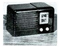
MODEL 40X30—Miniature 5-tube radio equipped with magic loop antenna; has automatic volume control; a.c.-d.c. operation; provision for victrola; electro-dynamic loudspeaker; beam power output; housed in walnut finished plastic case. Model 40X31 has all features described above, but, is housed in finished ivory. RCA Mfg. Co., Camden, N. J.
