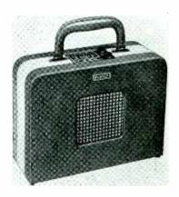
PORTABLE—Operates on a.c., d.c. and battery; uses 5 tubes, loop antenna, automatic volume control, airplane dial; housed in flat carrying case with simulated leather finish. Available in 2 types; model 545 tuning from 170 to 555 meters and model 5455W tuning 15 to 55 and 170 to 555 meters. DeWald Radio Mfg. Corp., 440 Lafayette St., New York, N. Y.
