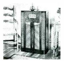
CONSOLE MODEL BK-42—Superheterodyne bat-tery receiver using 6 tuned circuits, one i.f. stage and magnetite core i.f. transformer. Has Econ-omy Blinker signal light to insure against needless battery drain; may be converted to a.c. house current; sturdy cabinet of two-tone heart walnut veneer, trimmed with zebra wood; measures 371/4" high, 24" wide, 111/9" deep. RCA Mfg. Co., Camden, N. J.
