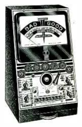
GIANT TESTER—Model 325 tube tester with large rectangular 9 inch meter indirectly illuminated by two 6 volt bulbs. Complete range of filament voltages from 1.5 to 120 volts. Tests loctal, single-end, bantam, midgets, ballasts, gaseous recti-fiers and Christmas tree bulbs. Individual toggles test each element separately. Line adjustment, short and leakage tests, headphone jack for noise tests. Simpson Elec. Co., 5216 Kinzie St., Chicago, Ill. Chicago, III.
