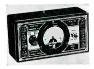
TROUBLE TRACER—Model 456 accurate inexpensive pocket size general utility instrument. Voltage ranges from 5 to 1000 volts; resistance from 5000 to 500,000 ohms; two current ranges of 0-1 and 0-10 ma.; decibels from minus 12 to plus 54. Radio City Products Co., 88 Park Place, New York, N. Y.
