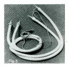
been proven by extensive usage, and for mechanical wearing qualities, the ordinary 7 mm. cable appears to be fully as satisfactory as most well made test leads. But in order to avoid eventual wire strand breakage due to excess handling of the test leads, an effort should be made to obtain 7 strand chromium steel 7 mm. ignition cable. It is virtually impossible to break any of these strands by ordinary flexing.
