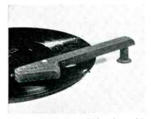
CRYSTAL PICKUP—Model X-79A phono pickup with convenient single mounting hole fastener; may be used on motorboards 1/16 to 1/2 inch thick. Frequency response stated to be 50 to 8500 cycles; 2.5 ounce needle pressure. Arm assembly is rubber cushioned eliminating micro-phonic feedback and motor noises. Available with or without built-in pilot light. Webster Electric Co., Racine, Wisconsin.
