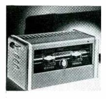
AMPLIFIER — Model 2418-A, an 18 watt unit adapted to general public address requirements. Has two inputs and tone control, output impedance is variable. Uses 7 tubes, transformers are well impregnated and wiring is cabled using flame-proof wire. Erwood Sound Equipment Co., 224 W. Huron St., Chicago, III.
