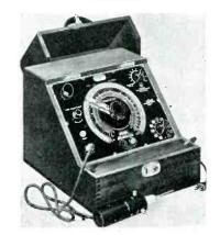
EXAM-ETER — New circuit and component analyzer. Serves as output indicator, dual range peak-voltmeter; r.f. alignment indicator; capaci-tance bridge; resistance bridge; power tactor in dicator; leakage indicator; and continuity checker. Solar Mfg. Co., Bayonne, N. J.
