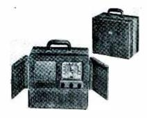
PORTABLE - Combination 4 tube battery with switch-over to 5 tube a.c.-d.c. portable with frequency range from 550-1720 kc. Loop antenna, 5½ in. P.M. speaker, avc, automatic shut-off switch cuts off current when doors are closed. Airplane linen case, 16½ lbs., weight. Radio and Television Retailing, July,
