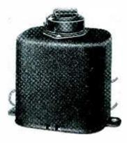
FILATROL-Model 767 unit can be used in conjunction with any early tubechecker for testing Loktal, Octal and other tubes having high filament voltages. Leads provided on unit connect to 110 volt ac outlet, 4-prong socket of checker. Switch then permits adjustments from 35 to 100 volts. Compact enough to fit spare compartments of portable tubecheckers or readily mounted on shop instru-ment panel. \$4.65. Radio and Television Retailing. July. 1939.
