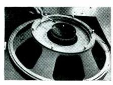
SPEAKING OF SPEAKERS—Giant 27 inch electro dynamic by Cinaudagraph handles up to 85 watts of audio. Look at the size of that voice coil compared to the pencil
