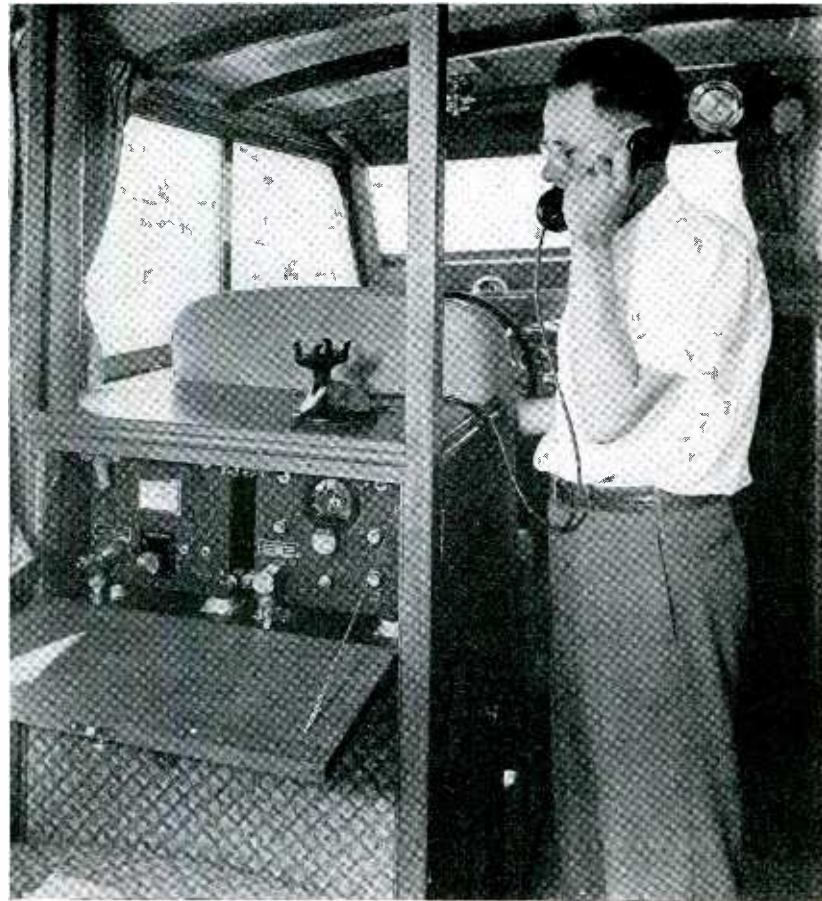
FIG. 5. Typical ship telephone installation on a 44 foot cruiser. Small transmitter sends signal to shore, receiver picks up shore signal, completing the circuit. Preset frequencies simplify operation.
