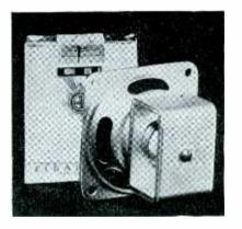
AMPHENOL—Molded sockets for bantam junior tubes such as HYII3, HYII5, HYI25 are available molded from high dielectric black bakelite or from ultra-low-loss mica-filled bakelite. Accommodates both 5 and 6 prong tubes. Sockets extend below the chassis only 1/16 in. more than the tube prongs, mount in plain round 5½ in. hole. Held firmly in place by retainer ring. No screws or rivets required. American Phenolic Corp., 1250 Van Buren St., Chicago, III.
