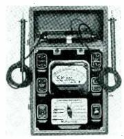
plify work by allowing meter to be used either for socket analysis or point to point testing. In use, connect multimeter to two pin jacks provided, two pin jacks provided, make necessary voltage and resistance tests between any two tube elements by pressing one button in upper row and one in lower corresponding to RMA numbered tube element. To take current measurements press. measurements, press same numbered upper and lower buttons and meter is automatically cut into
