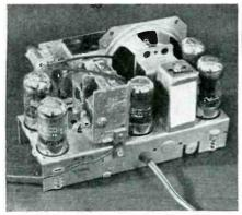
"LOKTAL" TUBES IN USE—Compactness is achieved in this typical chassis through the use of the new glass types (all glass except for metal base shield) by Philco
