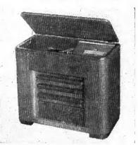
Model 739—A 7 tube a.c. superhet which covers tuning range in 3 bands 538 to 1750 kc., 2300 to 7500 kc., 7000 to 22000 kc. Ten inch speaker with automatic volume control, base compensated audio system, 6 button mechanical mute tuning. Phonograph attachment.
