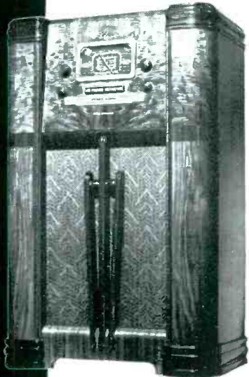
Model 91-512 —5-tube superheterodyne, with lighted dial, tone control, A.V.C., and new 4-station Magic Keyboard. Lighted dial covers 540-1720 kc. A really outstanding value.
