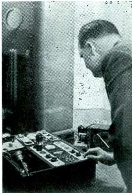
SECOND STEP —Next, tubes are tested, the chassis is removed and circuits aligned "right on the nose" . . .
