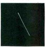
Pure 400 cycle sine wave as shown, left, gives straight line with number 2 connection.
