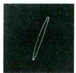
Same as left, but with pushpull connection. Unbalanced d.c. in transformer. Only slight difference between positive and negative peaks.
