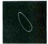
Wave distortion due to iron core saturation, too much d.c. in transformer. Note dissimilarity between positive and negative peaks.
