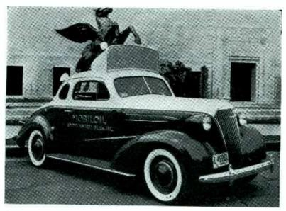
WINGED HORSE AND SOUND—Socony-Vacuum Oil's flying horse trademark can't be missed atop this promotion car sent to fairs, parades, calebrations. And beneath the horse is a neat housing for two Operadio speakers. In the rear computment of the cur is an Operadio mobile amplifier, complete with a gas-powered generator. Controls for the sound system are on the dash
