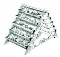
need of a place for small odds and ends. Since it is kept on the bench it permits easy access to the parts; also, as it is always before you, it tempts the serviceman to sort out the "chaff" that accumulates.
