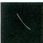
Wave distorted; plate loading resistance too low. Rounded negative (left photo) shows up as curved portion of line with number 2 connection.
