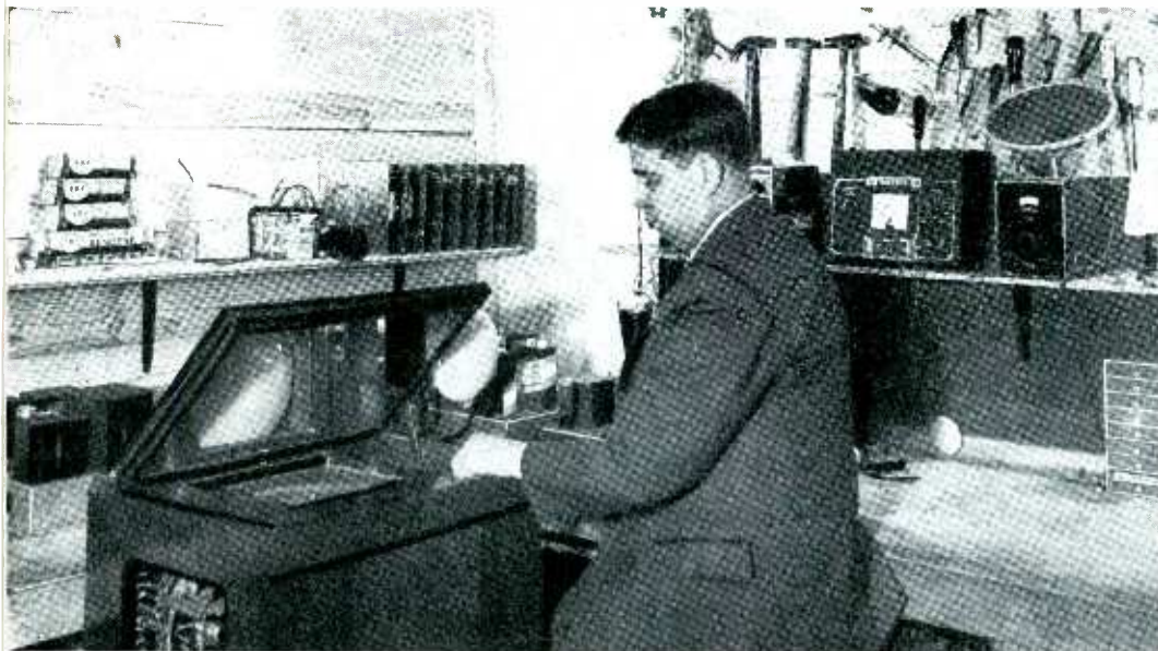
VIDEO TESTING —The author servicing a modern television receiver with the monotron oscilloscope shown below. The receiver is of British manufacture.
