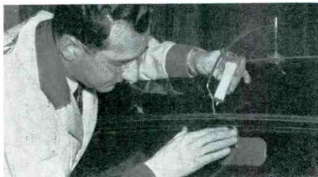
WATERPROOF STREAMLINERS —Lead-in wire under windshield raises rubber gasket, lets water drip inside. Fill openings each side of wire with flexible celluloid cement.
