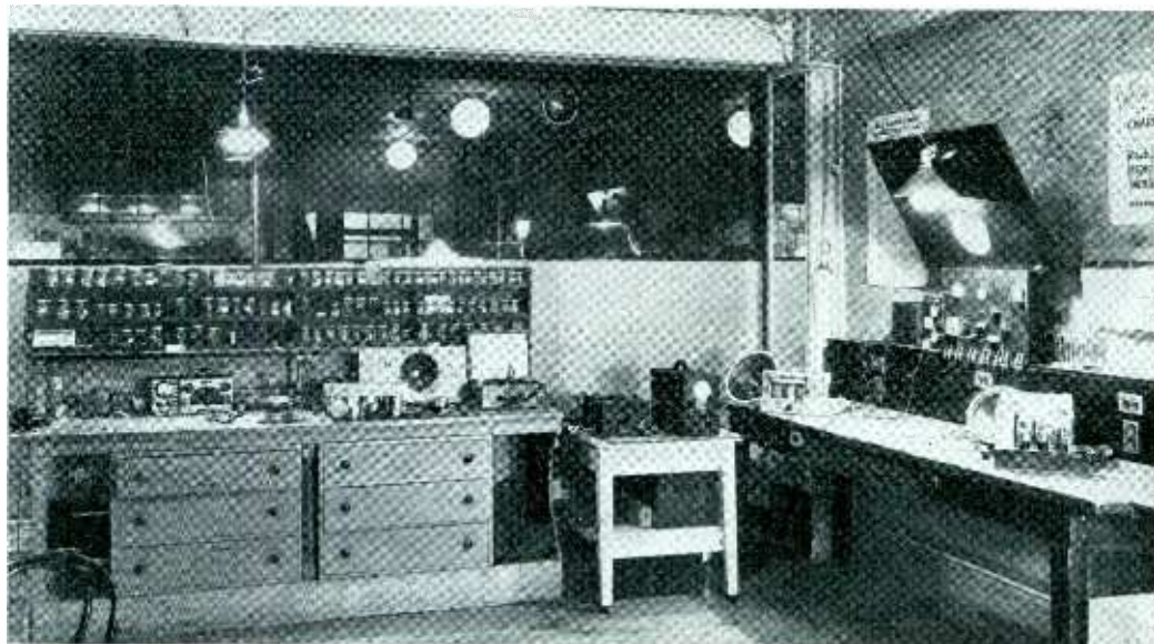
BOTTLE BENCH —Glass jars are a neat and effective way to keep small parts. This bench of Jackson Furniture Co., Oakland, Calif., is conspicuous by the absence of junk, dust and dirt.
