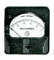
PANEL INSTRUMENT -- Illuminated dial of non-warping translucent material; bridge type construction and soft iron pole piece which, it is claimed, give it greater accuracy and added stamina; available in both dc and ac volt meters, milliam-meters and microameters, as well as thermo couple ammeters and milliammeters in all conventional ranges; mounts in a round hole 23/4 in. in diameter
