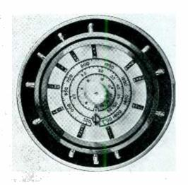
Stations are set on Sentinel by thumb screws on dial rim. Bottom pin is condenser stop.
