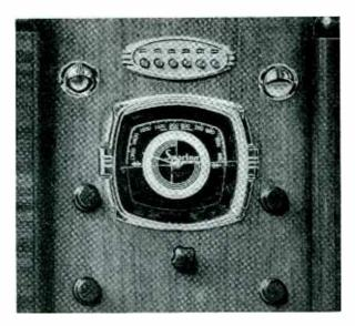
Capacity selector of Sparton, tunes independent of main tuning dial.
