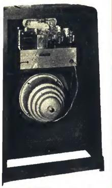
INDIVIDUALITY . . . Over the back of the speaker in this receiver is a cover comprising two concentric sections, plainty visible to the consumer. Low frequency response may be adjusted to fit rooms by varying the rings
