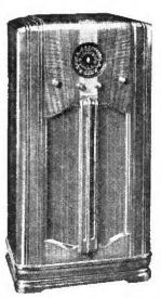
MODEL 650 — 6 tube, 9 tube performance Console for AC operation. American-Foreign-Police 3 Band improved superheterodyne. Range: standard broadcast 540 to 1500 Kilocycles; police and short wave 1500 to 4500 Kilocycles; short wave 5500 to 16500 Kilocycles.
