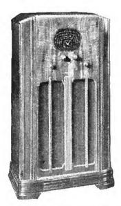
MODEL 6705 — "Automatic Maestro" model; 9 tube, 11 tube performance, All-Wave American, Police and Foreign, plus U. S. weather band, improved superheterodyne Console, Range: standard broadcast and police 525 to 1800 Kilocycles; police and short wave 1800 to 6000 Kilocycles; short wave 6000 to 18500 Kilocycles; and long wave U. S. weather band 150 to 375 Kilocycles,
