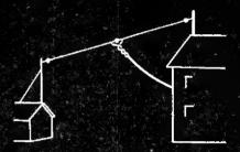
SIMPLE DOUBLET—Reduces noise pickup by downlead where it must pass through noisy areas. Good reception on shortwave band and satisfactory for broadcast reception. Especially afficient at certain frequencies, which may be those most offen desired.
