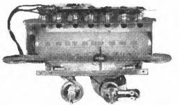
COLOR . . . Here is the first published shot of a floodlighted dial that glows red between stations, fades smoothly toward white as resonance is approached, turns brilliantly green when the signal is tuned right on the nose.
