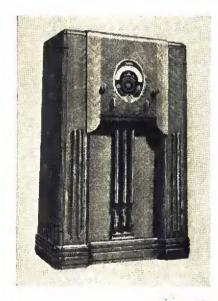
Model 91-C-4: Turret-Shield-ed,9-tube super-beterodyne with Tone Projector. Oversize, Turret-Shielded chassis. Metal tubes. Semaphoredial. Tunes American and foreign stations, police, aviation, and amateur conversation. Tuning range, four bands, including ultra short-wave. Dimensions: 421/2 in. high; 261/2 in. wide; 131/8 in. deep.
