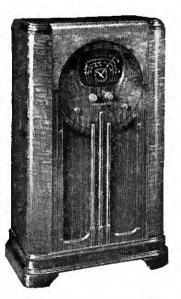
MODEL 670C — "Automatic Maes-tro" model; 9 tube, 11 tube per-formance, All-Wave Ametican, Police and Foreign, plus U.S. weather band, improved superheterodyne Console. Range: standard broadcast and police 525 to 1800 Kilocycles; police and short wave 1800 to 6000 Kilocycles; short wave 6000 to 18500 Kilocycles; and long wave U.S. weather band 150 to 375 Kilocycles.
