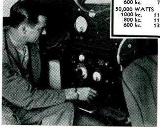
THE AUTHOR...with the mobile field-strength measuring instruments used in a recent survey for Station WOR. He drove 6,436 miles, took over 800 readings
