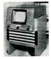
This German sight and sound receiver is claimed as simple to operate as an ordinary set. One tuning dial, adjusted for sound reception, automatically adjusts for best picture repro-production. Knob at right regulates picture for brilliance. Left knob for sound volume.
