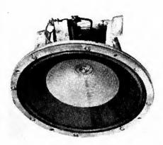
HIGH-FIDELITY SPEAKER used with the clarifiers described above. It uses an aluminum voice coil, whose mass responds readily to high frequencies, and a heavyand-thin paper composite cone
