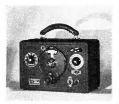
Standard all-wave test oscillator employed in conjunction with basic unit and frequency-modulator when aligning, checking intermittent reception, comparing overall receiver performance
