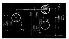
use of four tubes in place of the three diagrammed.
