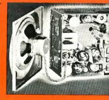
Heavy - Duty Tone - Matched Speaker built in front cover of single-unit models. Comes out with front cover, exposing radio chassis, without taking set from car.
