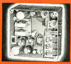
Standardized Chassis Design— All three models in metal case of the same size. Tables and other parts exposed for service by removing the front cover. Model 27 chassis above.
