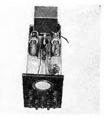
Basic oscillograph unit equipped with built-in vertical and horizontal plate amplifiers plus necessary half- and fullwave rectified power supplies
