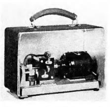
Motor-rotated condenser type "frequency-modulator" accessory needed only for alignment work
