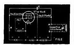
control or input element produces an increase in a.c. plate current, hence a decrease in a.c. plate voltage due to resistive drop in the load. Thus voltage changes in input and output are out of phase.
