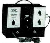
Reads sensitivity in approximate microvolts — Complete attenuation at all frequencies—All wave vernier tuning from 100 K.C. to 10,000 K.C. fundamentals—Separate 400 cycle available—Individually hand calibrated — Fully A. C. operated not A. C. - D. C. — Modulated 40% at 400 cycles—Output of 500,000 microvolts to zero — Portable zero
