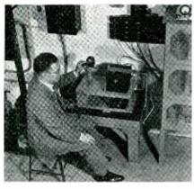
This device "jiggles" a-r sets 3,425 times a minute and is Emerson's "proving ground" whereby "the severity of a five-hour test exceeds that of 30,000 miles of hard driving," according to John B. Hawkins, its designer and operator.
