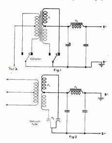
or other insulating material between the closed contacts of the vibrator. Otherwise you may have the delightful experience of checking all the way through the circuit only to find that the "short" is caused, quite normally, by the closed contacts of the rectifying vibrator contacts across the transformer secondary. (Fig. 1.)
