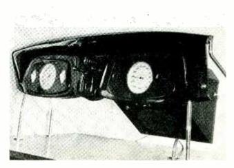
FORD DASH + What the well-dressed Ford dash looks like. Of course its embellished with a radio set. Note the open-face dial to match speedometer and the built in tuning panel
