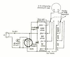
using for the past six months with excellent results. Using a 5 mil. meter with 35 ohms internal resistance it is possible to measure from 1 ohm to 2 megohms, in four ranges. A more sensitive meter and more taps on the switch would exceed this range but it would probably be necessary to use a special switch with less contact resistance.
