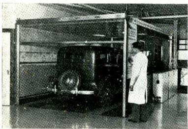
Valued as a prestige and publicity builder as well as for its technical merit, is the copper screened "radio cage" constructed by the employees of the P. J. Durham Company, Inc., New York City. In this room, entirely protected from outside electrical interference, motor car radio installations are given the final once-over. Even the floor
