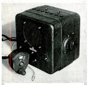
MODEL C-41—Four-tube set combining 7-tube performance with low battery drain. Full, brilliant tone even in high registers. Automatic noise suppression that cuts out , indistinct signals. Factory-sealed vibrator (guaranteed for 90 days) replaces rectifier tube. Increased output gives ample volume. Broader range—gets more daytime programs. Automatic volume control. Two-point tone control. Illuminated dial. Easily installed—only one mounting stud required. Fits all cars. Furnished complete with
