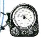
This oversize, illuminated dial on steering column is graduated in kilocycles. Easy to tune. Pilot light shows if set is on. Removable shutoff plug locks reInlies unless this ! as point of original
