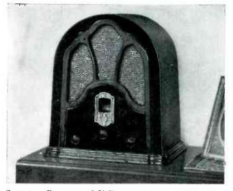
GENERAL ELECTRIC J-70 TABLE MODEL-A new cabinet style in full-size table models. An improved 7-tube superheterodyne with 2 super control tubes and Pentode output. Floating chassisrubber mounted. Full range tone control. Dynamic speaker. New, distinctive two-tone cabinet with beautiful glossy finish. Instrument panel finished in dark burled walnut. Dimenwith tubes sions 17 1-4" high, 14 3-4" wide, 10 1-4" deep.
