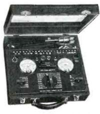
The Jewell Pattern 444 Set Analyzer allows rapid servicing of receivers employing even the most complex circuits.
