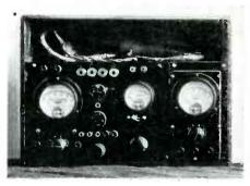
method of voltage reading is that the voltages between any tube element and the grounded chassis can be obtained by clipping one of the leads to the chassis and inserting the other in a tip jack. I have found this particularly useful in the case of modern circuits incorporating isolating resistors in grid and plate circuits and variable grid biases. A chassis to plate reading is more reliable in such cases than grid to plate or cathode to plate check.
