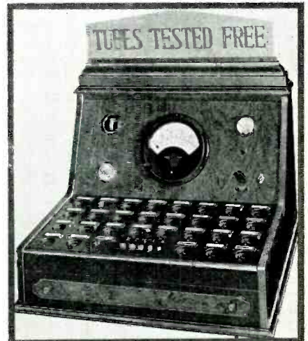
Jewell's model 536 operates on the "grid-shift" principle in which plate current readings are taken at two points on the grid-voltage plate-current curve as a mutual conductance check
