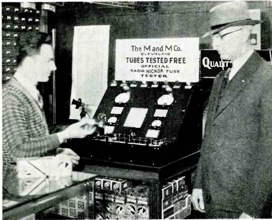
The Hickok type A.C. 4300 instrument illustrates a modified "a.c. output" type, using a plate circuit a.c. meter calibrated to indicate mutual conductance directly in micromhos when standard signal is applied to grid
