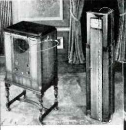
HERE'S THE LONG BAFFLE. The shorter the baffle, the fewer low tones you hear. Notice the difference in baffle in standard style cabinets (left) and the "Columaire" (right).
