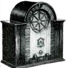
AC MODEL: 2-P224 Screen Grid TRF,1-P224 Screen Grid Power Detector, 1-P227 1st Audio.1-P245 Audio Output, 1-P280 Rectifier.
