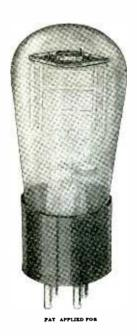
Armored bridge advantages are manifold. Improved spacing of tube elements insures greater uniformity and strict maintenance of operating characteristics. Shockproof, ultra-rigid mounting eliminates damage in transit and from rough usage. Perfect balance is assured by the elimination of the top-heavy bead construction, which contributed greatly to misplacement of elements.
