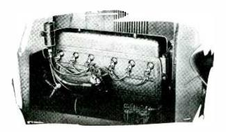
Seven 25,000 resistors, six at the plugs and a seventh in the center distributor lead, effectively suppressed ignition noise in this Chevrolet. When disturbance persists it is sometimes found that innocent looking chokerods, oil-gauge tubing, metal cable coverings are acting as conductors for the offending high-frequency currents. Run the motor, hood closed, and short suspected parts to chassis with a screwdriver. (Delco)
