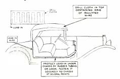
Installation of sets which are not designed to use capacitor plate antennas in open cars necessitates the design of a "false top" type of antenna and the exercise of considerable ingenuity in concealing and fastening the "grid" arrangement illustrated (Crosley) in the top. The wire used must be stranded and sufficiently flexible to fold with the top without ill effect.
