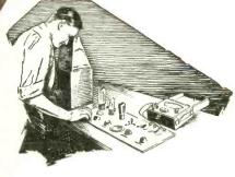
The Oscillograph tests Y-227 tubes for "hum." It is one of the devices by which the Hygrade Quality Department makes sure that the Red Triangle trade mark means "Tubes You Can Trust."
