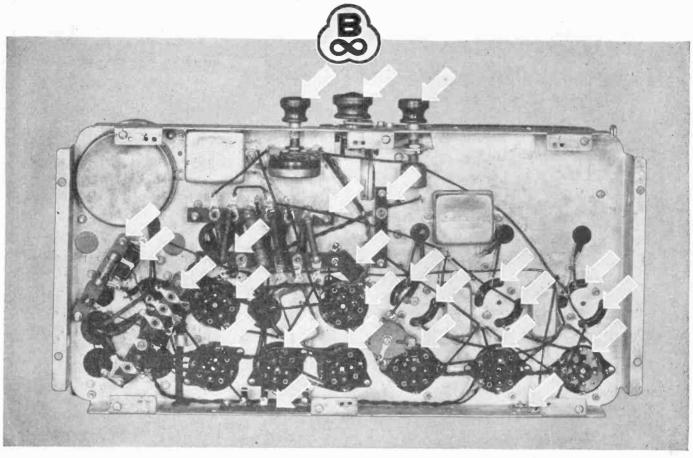
Chassis of The Crosley Unitrad Receiver, with Bakelite Insulation indicated by arrows. Made by The Crosley Radio Corp., Cincinnati, Ohio.
