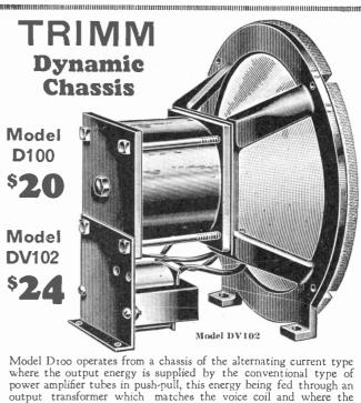
where the output energy is supplied by the conventional type of power amplifier tubes in push-pull, this energy being fed through an output transformer which matches the voice coil and where the power pack supplies direct current for energizing the field coil.
