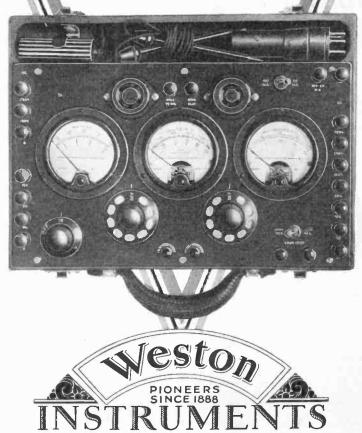
D. C. Milliammeter—Double range—100/20 M. A. provides for lower readings with better scale characteristics.
