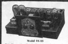
This Pierce-Airo Chassis fits any standard console. Note its compact and sturdy construction. The chassis also houses the self-contained power supply.
