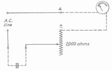
Circuit used for testing condenser capacity
