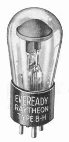
Eveready Raytheon BH Rectifying Tube— standard for "B" Power Units 125 m.a., 300 volts
