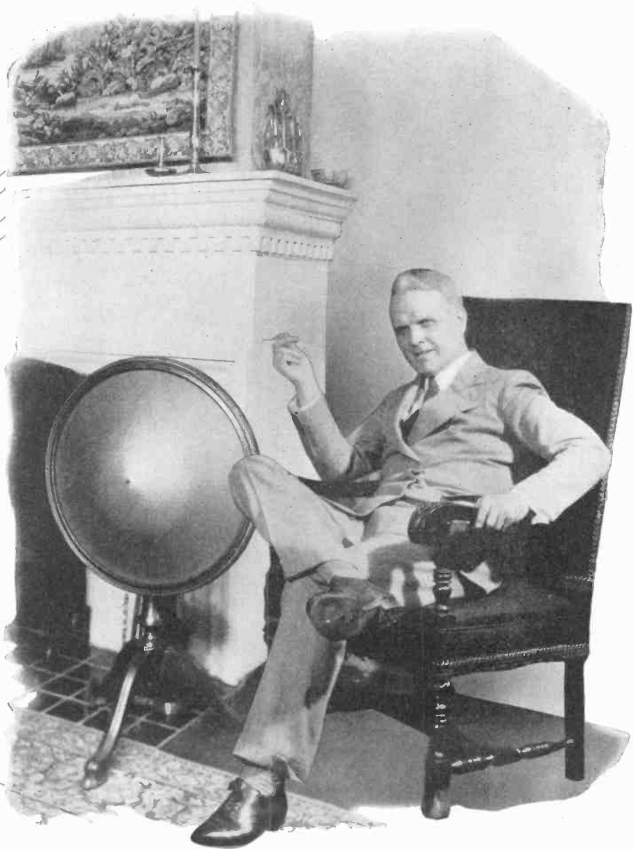
The customer simply has a speaker like this in the home. This plugs into an outlet connected to the distribution system over which come the programs.
