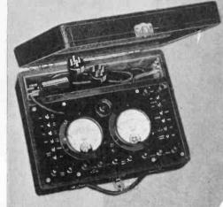
The Jewell No. 210 is the first tube tester to give direct readings, thereby eliminating mental arithmetic. It provides for variations in line from 100 to 130 volts. Tests all tubes. A 100 milliampere scale is provided for rec-tifier tubes. Gives individual teading of each plate of double wave rectifier tubes. Operates from A.C. service line
