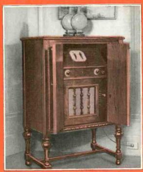
RADIOLA 30A.—Custorn-built cabinet model of the super-selective RCA Super-Heterodyne with loud-speaker. For either AC or DC operation from lighting circuit.
