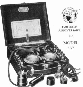
This new instrument provides for every required test in connection with the installation and proper maintenance of radio receivers. It will measure the various currents and voltages employed anywhere in the set, including those at the tube sockets. All tests can be made by using the regular voltages normally supplied to the set by its batteries or socket power without the necessity of changing connections. Nor is any auxiliary power required.
