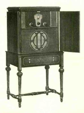
The model illustrated is the Kolster full console 6 tube electric set. Cabinet of walnut with special built-in cone speaker. This set operates from any 110 volt 60 cycle electric line. The tubes used in this set are as follows: four UX 226 or CX 326, one UY 227 or C 327, one UX 171 or CX 371, one UX 280 or CX 380. Price, \$250. Tubes extra.
