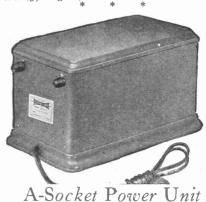
The illustrated Model A-7-A power unit, known as "Bone-Dri," made by the Webster Company, 3504 West Lake Street, Chicago, Ill. This supplies six volts at 12 amp, and uses 2 Raytheon cartridges for full wave rectification. There is also a receptacle in the unit where the B-unit may be connected, placing everything under the control of the filament switch on the receiver. The intended retail price complete is \$37.50.
