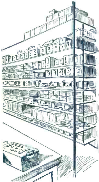
Waste space due to excess spacing between shelves is reclaimed by making alternate shelves half width as shown above.
