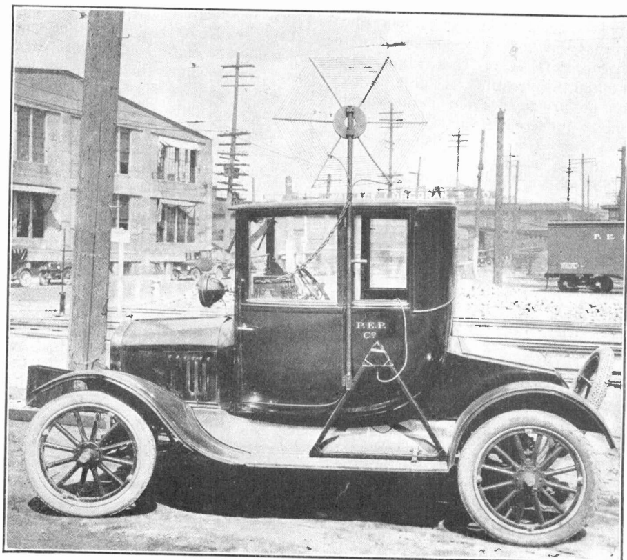
The Portland Electric Power Company, Portland, Ore., is doing excellent work in tracing down and eliminating interference with radio reception in the section around Portland. By means of the radio-equipped auto pictured above, it is possible to find the exact location of the disturbing noises.
