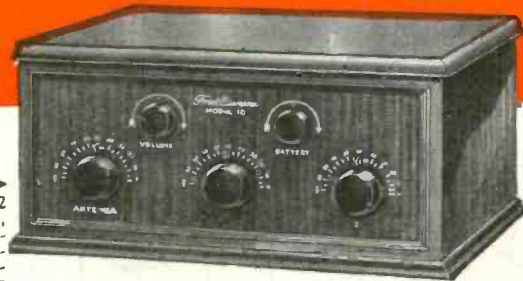
Model 10*—5-tube set, 2 stages tuned radio frequency, detector and 2 stages transformer coupled audio frequency amplification. Battery cable provides for power tube. List price $60.00.
