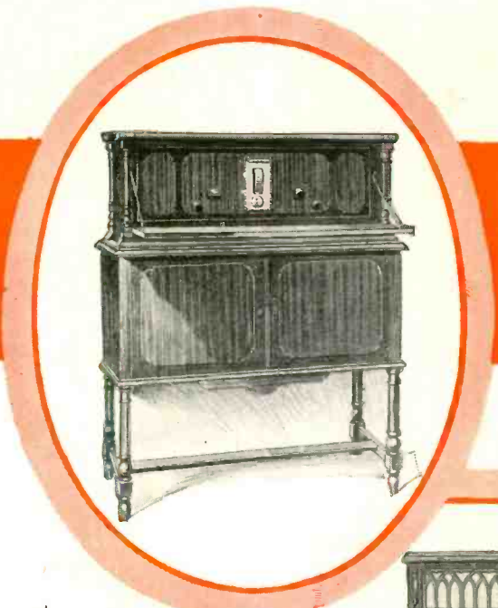
↑ Model 50* —7-tube, single control receiver. 3 stages TRF amplification, detector and 2 stages transformer coupled audio frequency amplification. Chassis of pressed steel; partial interstage shielding. Battery cable, wired for use with new detector and power amplifier tubes. Wavelength scale visible through indicating window. "A" battery voltmeter mounted on the 5-ply two-tone mahogany front panel. Antenna compensator is provided for DX tuning. List price $175.00.
