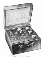
The Superadio Dynometer matches tubes and gives the dynamic characteristics, without calculations and without error.
