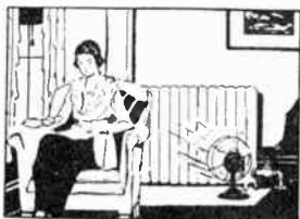
Fan increasing Heat Radiation of Sluggish Radiator
