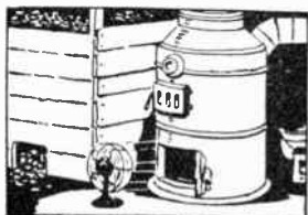
Fan used to improve Furnace Draught
