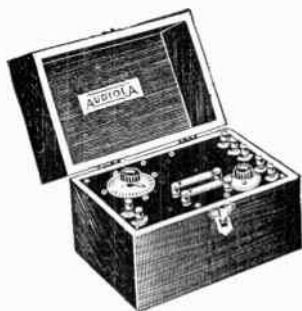
Vacuum Tube Receiving Set —The "Audiola" vacuum-tube receiving set was developed, according to its manufacturer, to supply the demand for a high grade, reasonably-priced vacuum tube receiving set having a range of from 300 to 600 meters. Only two adjustments are necessary in operation.—Audiola Radio Company, 430 South Green St., Chicago.
