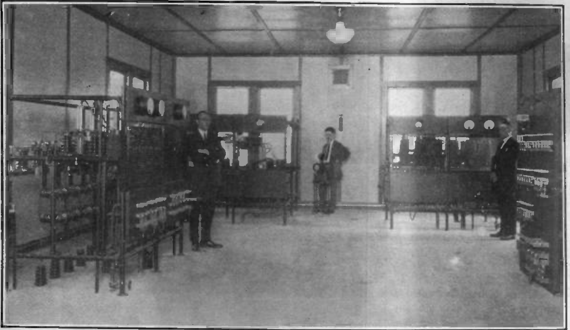
Fig. 7. On the Left of This Picture of KDKA May be Seen the Sets of Water-Cooled Tubes Like Fig. 4; Also the Coils of Hose.
