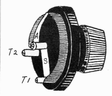
Fig. 3. Here is a Place Where High Resistance Wire is Needed.
