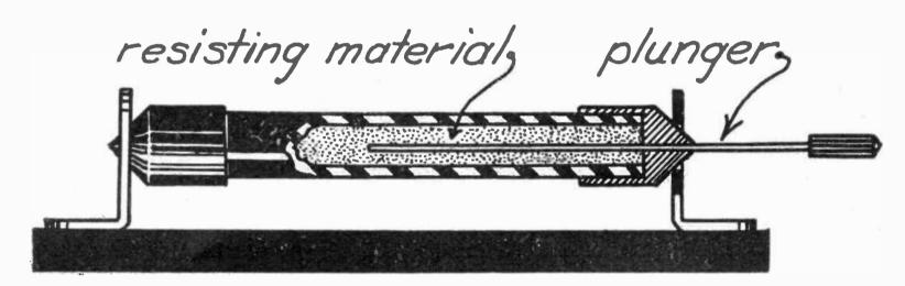
Fig. 6. The Basic Principle of Most Variable Leaks
