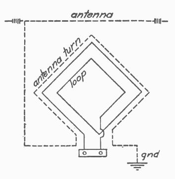
Fig. 1. By Combining Loop and Short Antenna, One Way Only is Picked Up.
