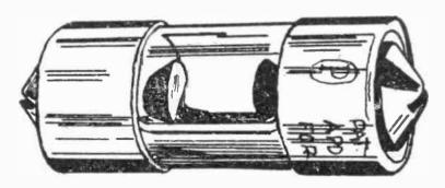
Fig. 8. The Liquid in Tube Touches More or Less of the Half-circle Ends
