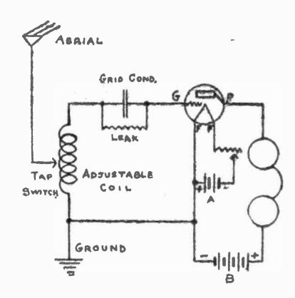
Fig. 1. This Hook-up Shows How Leak is Connected
