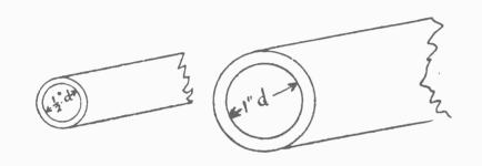
Fig. 1. Twice the Diameter Gives One-fourth the Resistance for Water or Electricity.
