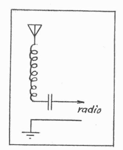
Fig. 3. This Acceptor Circuit Allows Only the Wanted Signal Through.
