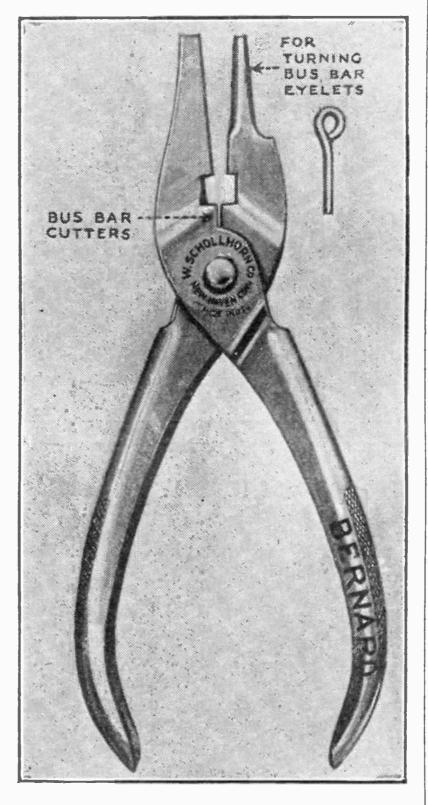
Fig. 2. Special Pliers That Will Make an Eye on the End of Bus Bar
