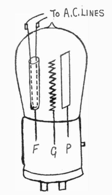
Fig. 2. Here is the Principle of the A. C. Vacuum Tubes
