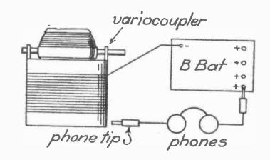
Fig. 2. How to Test an Instrument for Leakage.
