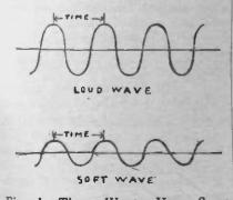
Fig. 1. These Waves Have Same Frequency But Different Loudness local wave without being disturbed. The better the set the narrower the band over which the local is picked up. However, even with the most expensive sets, you will find that the long distance work in large eities is done mostly after the nearby stations have signed off for the night.
