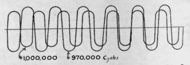
Fig. 8. Two Waves of Almost the Same Speed Will Give Very Broad Tuning if From Same Station
