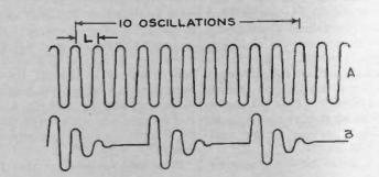
Fig. 4. Tuning for 10 Waves is Easy with Tube Sender, but with Spark It Can't Be Done
