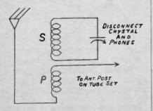
Fig. 5. Series Connection of Set Used as a Wave Trap
