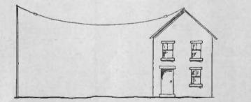
Fig. 2. With This Construction Your Signals Will Sometimes Fade
