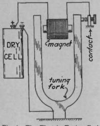
Fig. 1. The Electric Tuning Fork for Tuning Keeps Itself Running
