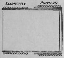
Fig. 3. A Scheme Like This Will Give Just the Right Coupling
