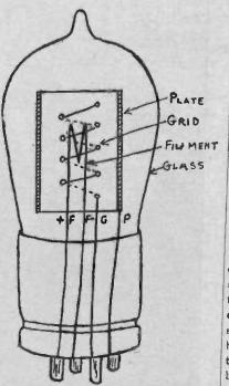
Fig. 5. The Construction of a Tube Affects the Internal Capacity from Grid to Plate.
