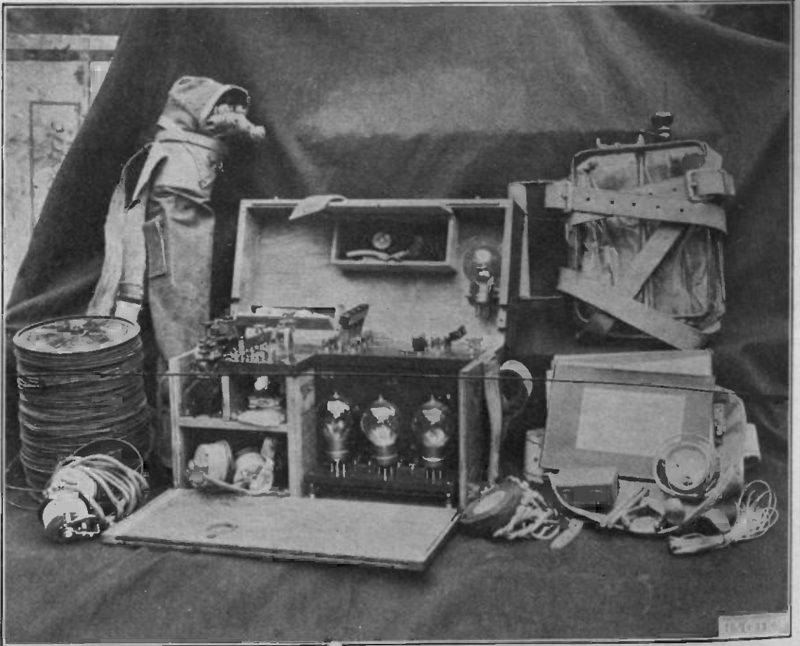
Fig. 2. This is a Combined Sending and Receiving Outfit. Three Bulbs and a Spare Carried.
