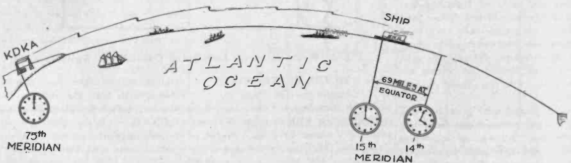
Fig. 1. Ships Depend on Correct Time to Know Where They Are. There is a Difference of Four Minutes Between Meridians.
