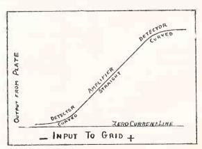
Fig. 7. This is the Curve Which Showas How a Tube Acts
