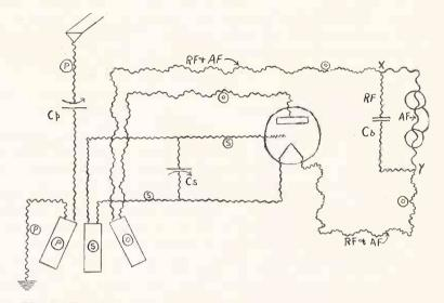
Fig. 3. This Shows the Path of Waves Through Wiring of Fig. 2
