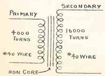
Fig. 1. Shows Principle of Iron-Cored Transformer
