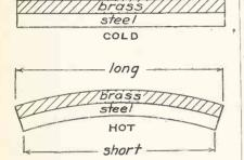
Fig. 1. Brass Expands with Heat and Bends Steel
