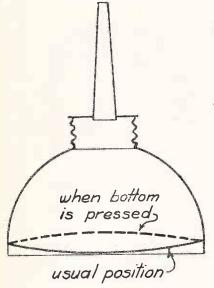
Fig. 3. Snap Action is Like Bottom of Oil Can
