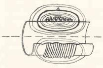
Fig. 1. A Honeycomb Coil is Like a Banked Winding Developed
