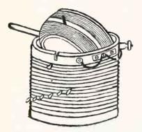
Fig. 3. It is the Taps on This Variocoupler That Count
