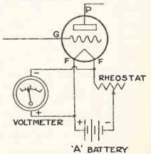
Fig. 1. Proper Way to Use Meter in Adjusting Filament
