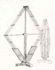
The superior construction of the DTW IMPORTED COLLAPSIBLE LOOP enables it to perform this function to much better advantage than other loop antenna devices. Forty-two inches high by forty inches wide, its inductance consists of fourteen turns of genuine Litzendraht cable, made up of sixty individual strands, insulated, twisted and covered with double green silk.
