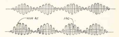
Fig. 5. How the Detector Treats the Amplified Waves of Fig. 4. Notice the Shape is Changed
