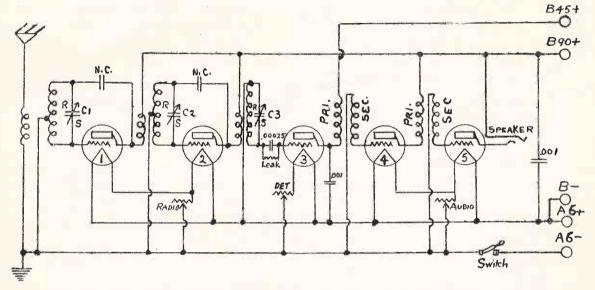
Fig. 6. Notice in the Left-hand Lower Corner the Connection from Ground to Filament Line. This Reduces Body Capacity
