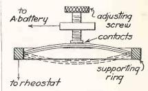
Fig. 4. How Contact is Made by New Thermostat
