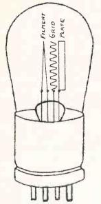
Fig. 6. The Necessary Parts Inside a Tube-Three Elements
