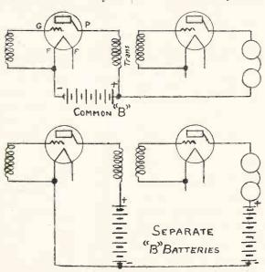
Fig. 2. This Invention Saves a Lot of "B" Batteries
