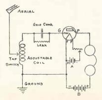
Fig. 2. This is a Very Simple Detector Circuit
