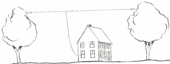
Fig. 3. Be Sure to Fasten Lead-in in Center of Flat Top—Not as Shown
