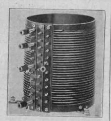
Fig. 7. The Antenna Coil. The Taps Are **Used** for Tuning
