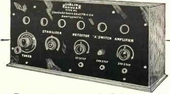
The set comprises two stages of radio frequency amplification, a detector and three stages of audio frequency amplification. The parts are mounted on a sub-base to which a Bakelite panel is attached. It is enclosed in a handsome solid mahogany cabinet.
