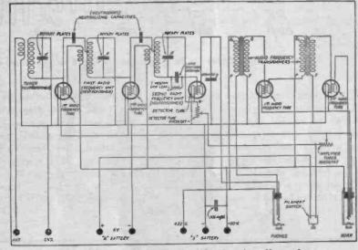
Fig. 4. Neutralized R. F. Amplification in a Neutrodyne
