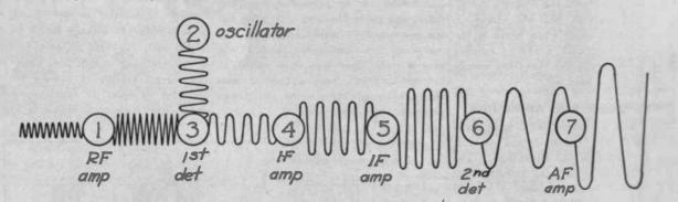
Fig. 5. What the Tubes Do in a Superhet. R. F., A. F., Detector, and Oscillator Tubes Are Needed
