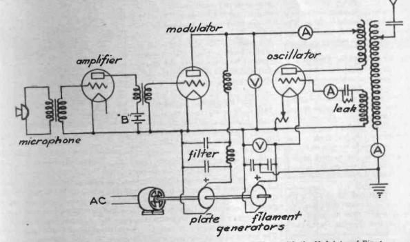
Fig. 6. Complete System. This Combines the Oscillator of Fig. 2 with the Modulator of Fig. 4
